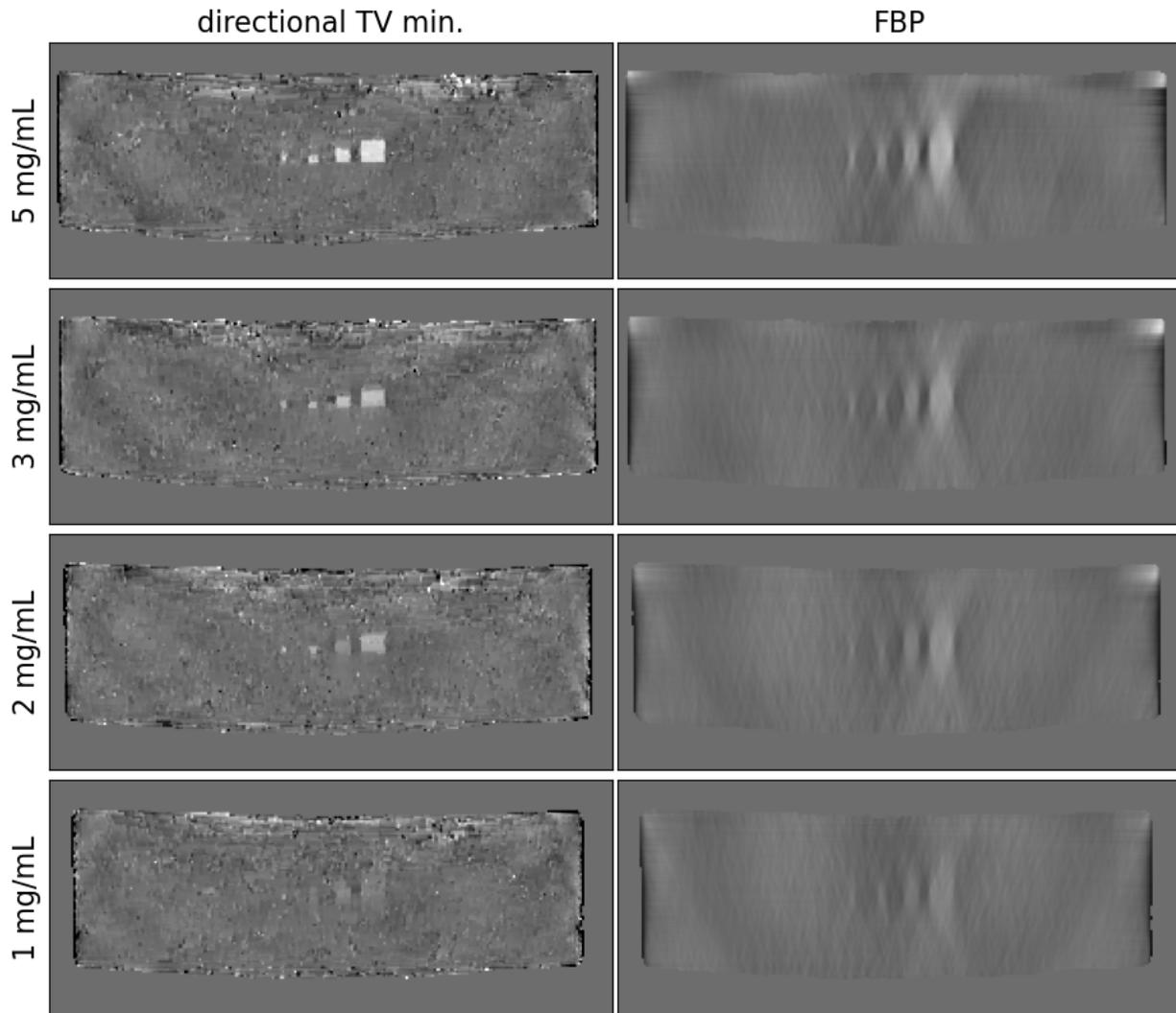
Fig. 4. Transverse plane images cutting through the groups of ICA objects of the same concentration with directional TV minimization and FBP images on the left and right, respectively. Concentration of the ICA decreases going from top to bottom. All gray scales are matched for quantitative comparison and the images are masked to the object support.
