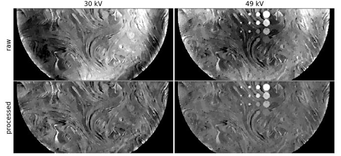
Fig. 2. Raw and processed in-plane images containing all ICA objects for the directional TV minimization images for the 30 kV (Left) and 49 kV (Right) DBT scans. Image processing is performed by polynomial fitting and normalization described in Eqs. (1) and (2), respectively. The gray scale for the raw images is selected to span the range of background variation, and the gray scale for the normalized images is selected to be  $\pm 30\%$  of background.
