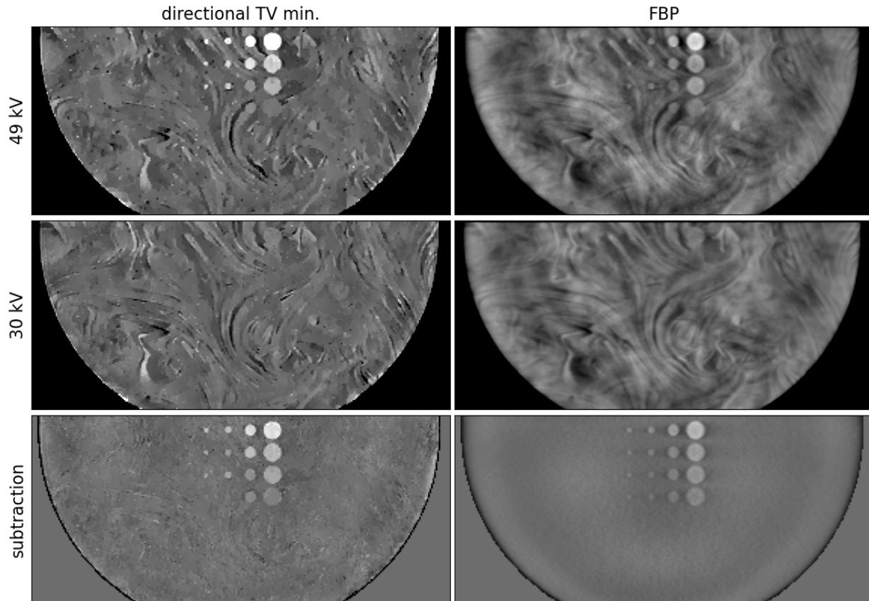
Fig. 3. In-plane images containing all ICA objects for directional TV minimization (Left) and FBP (Right). The top and middle rows show the images corresponding to the 49 and 30 kV acquisitions, respectively. The bottom row shows the weighted subtraction designed to isolate the ICA distributions. The gray scales on the left and right are matched and the images are masked to the object support.
