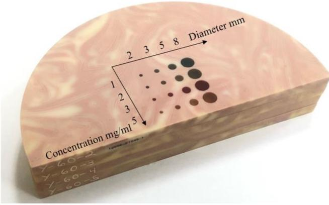
Fig. 1. CIRS phantom with solid ICA inserts. The background is heterogeneous with 50% glandularity.
