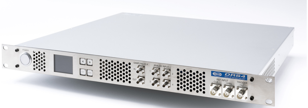
Figure 1. Front view of DRS4 customized for LMT-FINER. The LCD displays real-time power spectra and is used for device configuration together with four buttons on the side. The ANALOG INPUT port pairs 1/2 and 3/4 correspond to LSB/USB IF inputs for DC–10.24 GHz and 10.24–20.48 GHz, respectively. The SAMPLING CLK IN/OUT port receives/sends an external 20.48 GHz reference signal from the DRS4 Sampling Clock Distributor (Elecs Industry Co., Ltd.) for operating the four 20.48-Gsps ADCs. The REF INPUT 1PPS port receives an external 1 PPS signal for setting timestamps of the power spectra. Note that absolute date and time information should be given by an NTP server through the Ethernet port on the back panel. The Ethernet port is also used to output (multicast) the power spectrum data as VDIF. Other ports are not used in this model.
