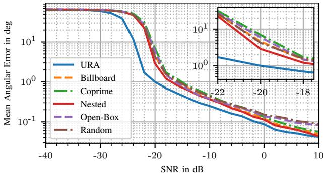
Fig. 9: Simulation across the angle space  $\varphi \in [0^\circ, 360^\circ]$  and  $\theta \in [0^\circ, 90^\circ]$  with  $K = 1000$  samples. The error metric is the spherical angles between estimation and the Ground Truth (GT) point.
