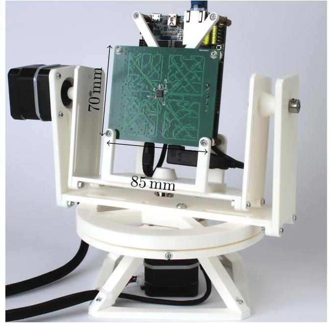
Fig. 6: The photo showcases the microphone array mounted on a two-axis rotation table<sup>1</sup>, essential for conducting accuracy measurements. Microphone capsules are situated on the back-side of the PCB, linked to the front side via dedicated holes. The PCB is sandwiched onto the Cyclone V FPGA board, which includes an Ethernet connection for data transfer and control.
