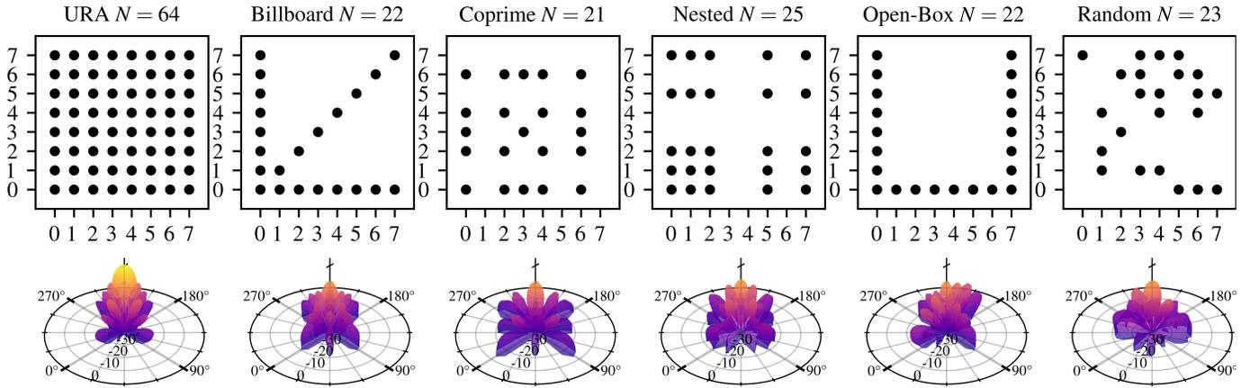
Fig. 8: The figure depicts the array geometries under investigation alongside their corresponding beam patterns as achieved with a classic delay-and-sum beamformer. The magnitude of the beam pattern is represented in dB and mapped to the radius.
