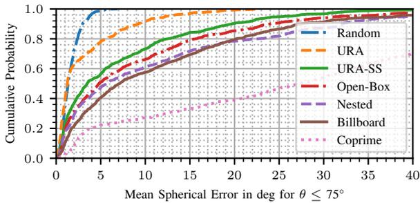
Fig. 14: The cumulative distribution function of the mean spherical error is computed with higher elevations  $\theta \leq 75^\circ$  excluded.
