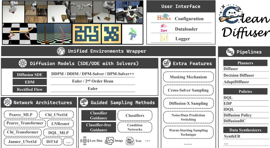
Figure 1: **The Architecture of CleanDiffuser.** CleanDiffuser is specifically tailored for the decision-making domain, supporting a wide range of Diffusion Models, Network Architectures, and Guided Sampling Methods modules and extra useful features. By simply combining the building blocks into a pipeline, CleanDiffuser integrates 9 popular DM algorithms.
