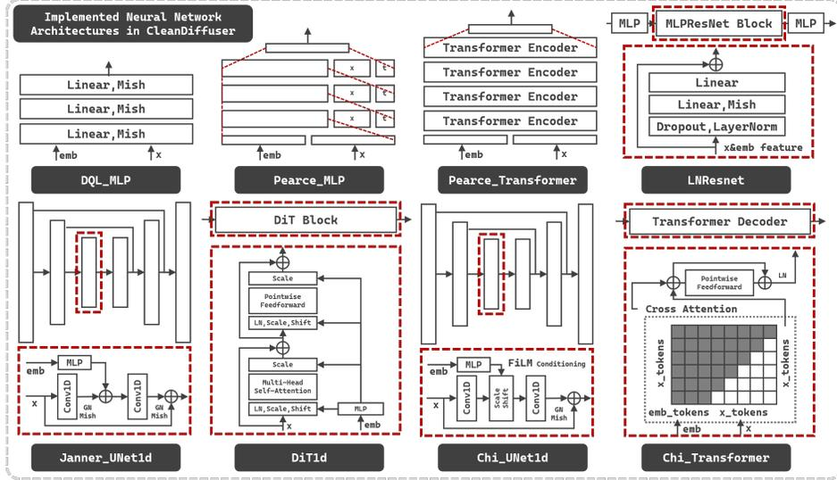
Figure 4: Visualization of Implemented Network Architectures in CleanDiffuser.
