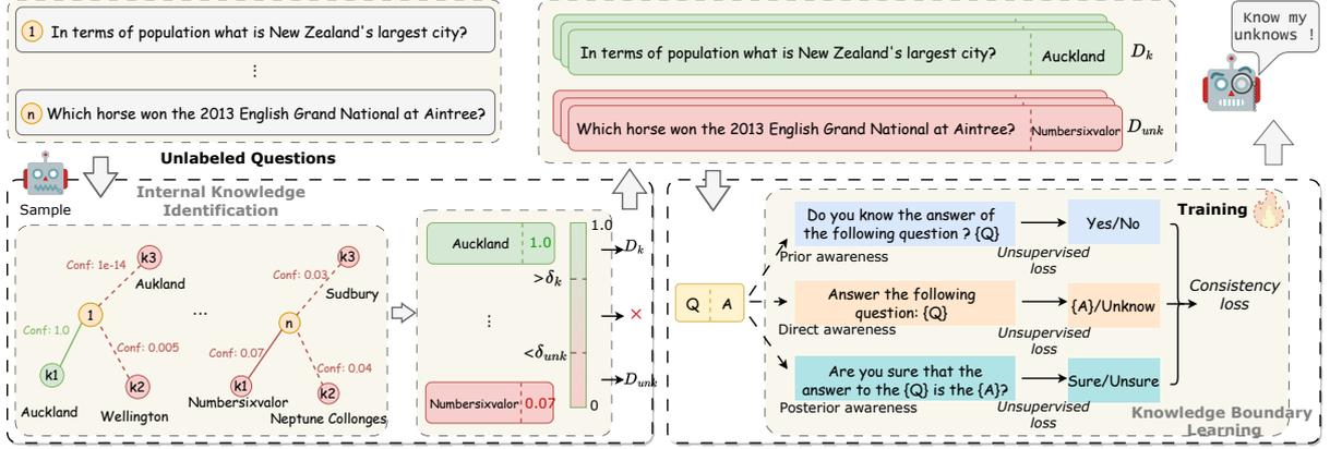
Figure 2: The procedure of CoKE, which consists of two stages. In the first stage, the model makes predictions for unlabeled questions. We obtain two parts,  $D_k$  and  $D_{unk}$ , based on the model confidence. In the second stage, we train with different prompts for the same question and use unsupervised loss and consistency loss to teach the model to express the knowledge boundary.
