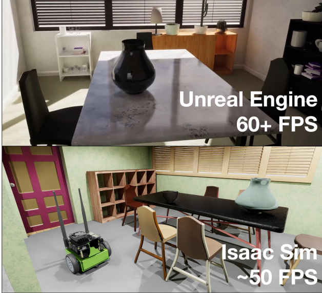
Figure 12. Two scenes imported into Unreal Engine 5 (above) and Omniverse Isaac Sim (below). Unreal Engine runs at 60 FPS, and Isaac Sim, with physics simulation enabled, runs at 50 FPS, both on RTX 4090s.
