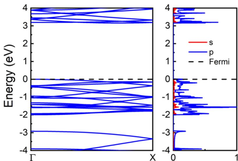
**Figure 3.** Band structure and partial density of states of penta-graphene nanoribbons calculated by the HSE06 hybrid functional implemented in the AMS package. The Fermi level is indicated by the dashed lines.
