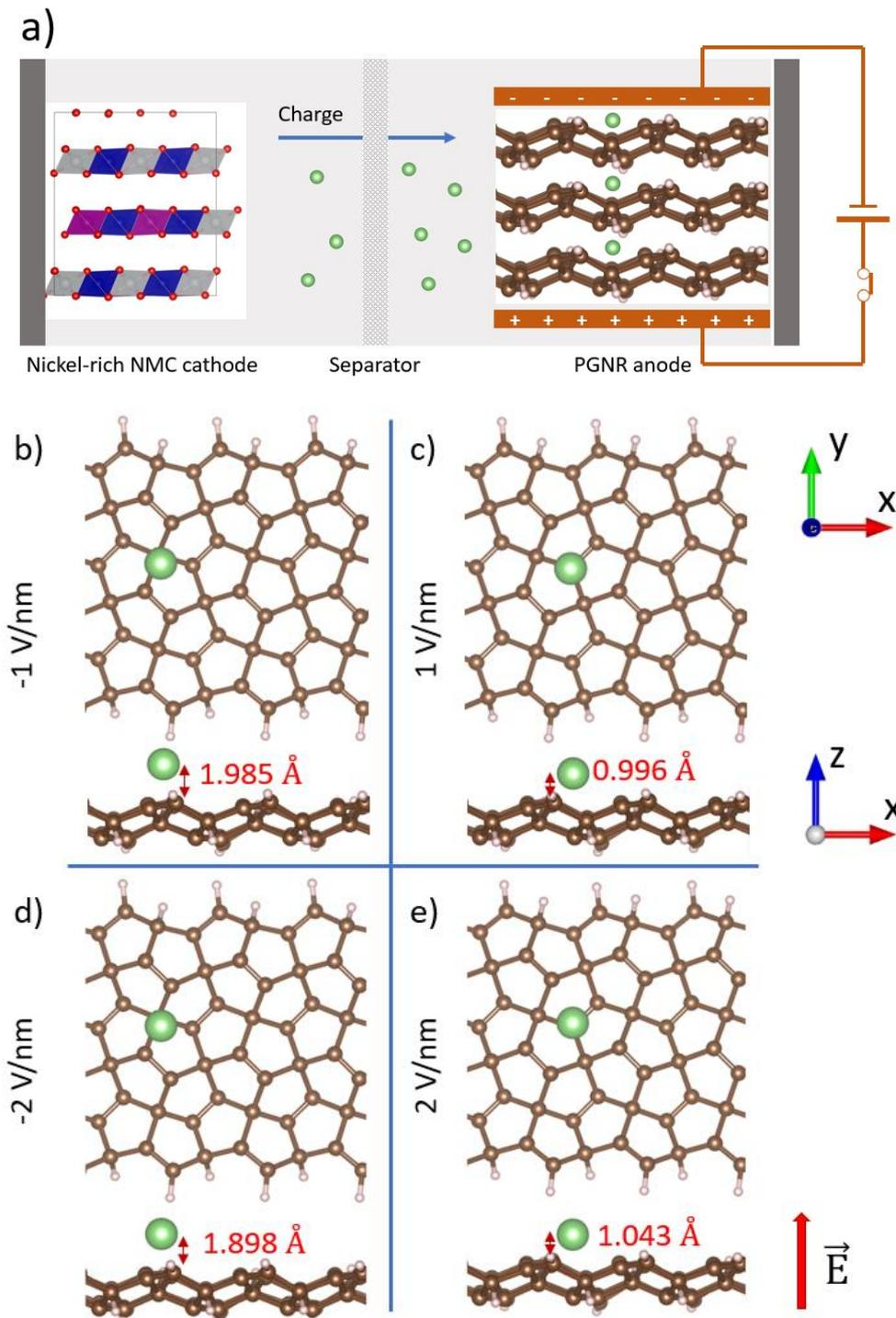
**Figure 2.** (a) Sketch of a lithium-ion battery with a penta-graphene nanoribbon anode under a vertical electric field. The geometrical structures with top and side views of these adsorbed system under an electric field of -1V/nm (b), 1 V/nm (c), -2 V/nm (d) and 2 V/nm (e). The positive direction of the external electric field is sketched at the bottom right of figure (e). The shortest distances from the adsorbed lithium-ion to PGNR are also displayed in these figures.
