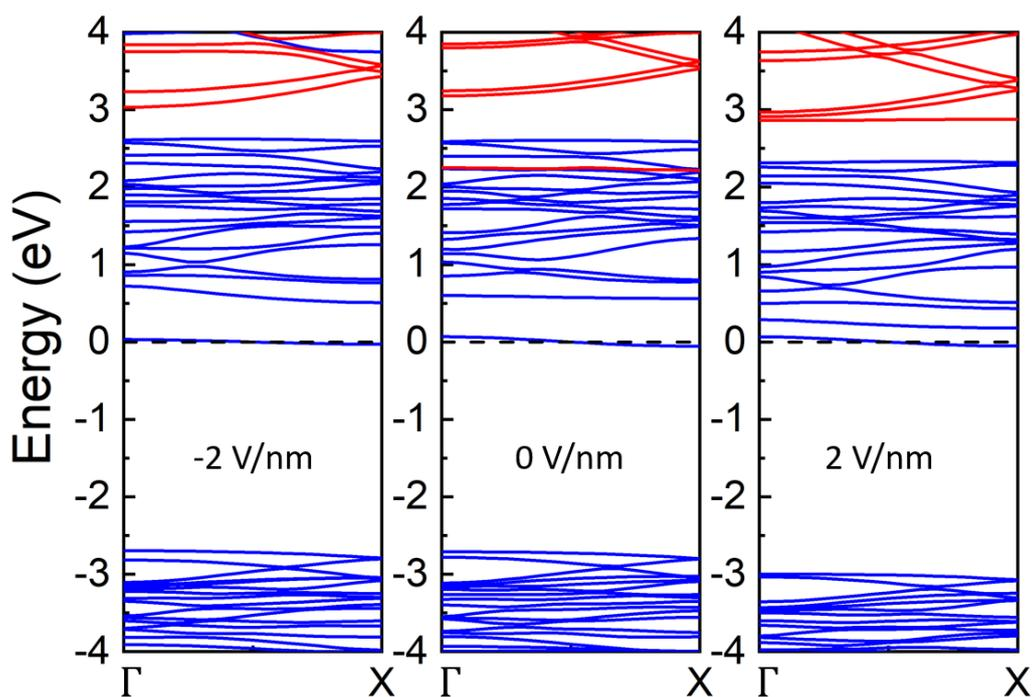
**Figure 4.** Band structure of penta-graphene nanoribbons upon adsorption of a lithium atom calculated by the hybrid HSE06 functional implemented in the AMS package. Red and blue lines represent for the s- and p-orbitals. The Fermi level is indicated by the dashed lines.
