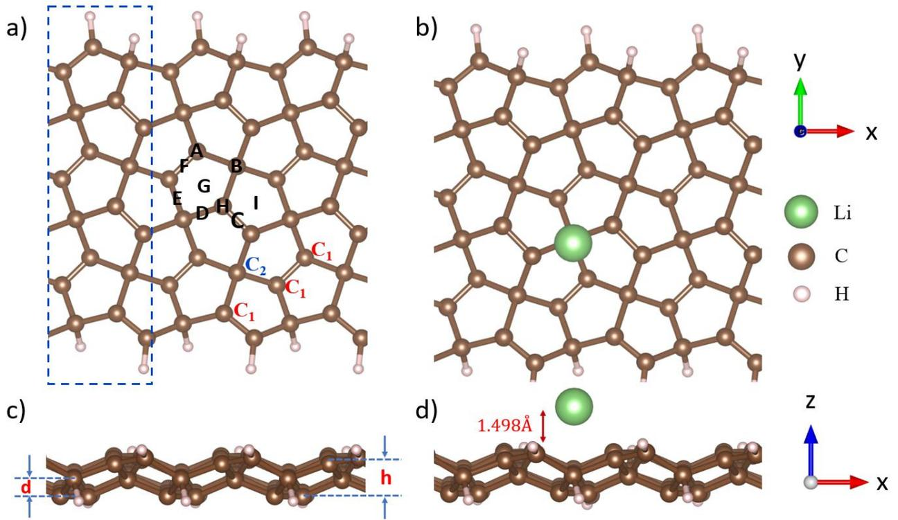
**Figure 1.** Top- and side-view of the optimized geometrical structures of PGNR (ac) and PGNR + Li (bd). The yellow, gray and white balls illustrate Li, C and H atoms, respectively. The possible Li adsorption sites (a) are marked as on top (A, B, H), at hollow (I, G), and in the bridge (C, D, E, F) of C atoms. The dashed blue rectangle represents the supercell of PGNR.
