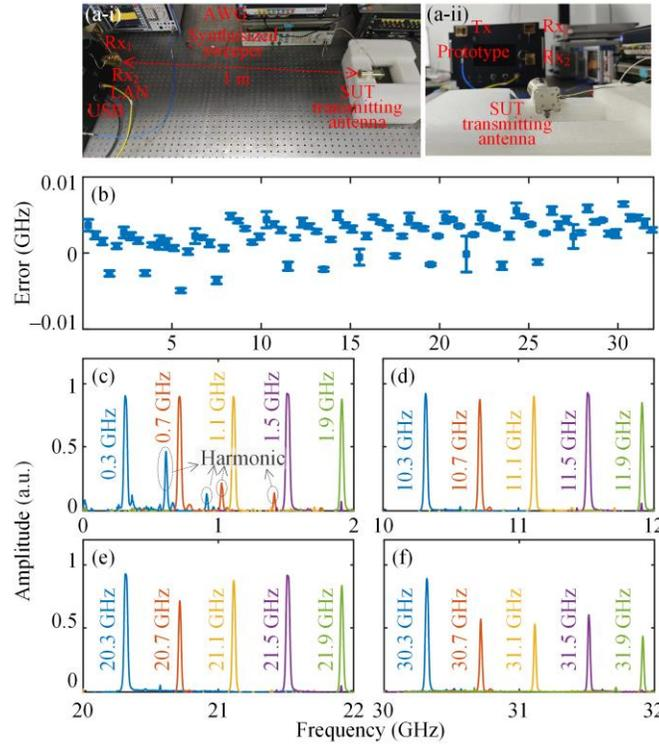
Fig. 9. (a) Photograph of the spectrum sensing setup. (b) Single-frequency measurement errors at different frequencies. Single-frequency measurement results when the frequency measurement range is (c) 0 to 2 GHz, (d) 10 to 12 GHz, (e) 10 to 12 GHz, and (f) 30 to 32 GHz.
