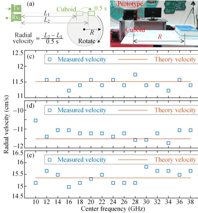
Fig. 6. (a) Schematic diagram of the radial velocity measurement. (b) Photograph of the radial velocity measurement setup. Radial velocity measurement results when the target rotates (c) clockwise and (d) counterclockwise with a rotation radius of 45 cm. (e) Radial velocity measurement results when the target rotates clockwise with a rotation radius of 60 cm.
