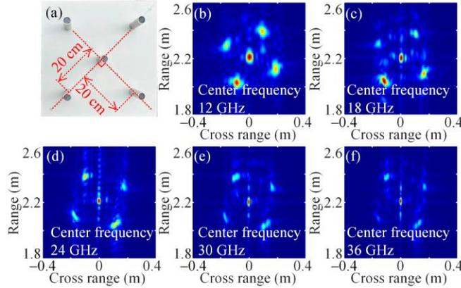
Fig. 7. (a) Photograph of five cylinders with an outer diameter of 3 cm for ISAR imaging. (b)-(f) ISAR imaging results obtained using the prototype operating at different center frequencies.
