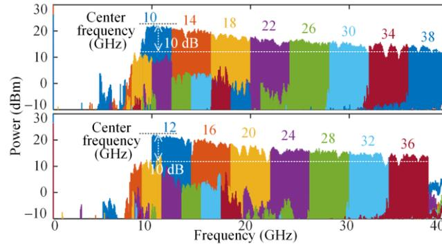
Fig. 3. Electrical spectra of the generated 4-GHz bandwidth LFM radar signal ranging from 8 to 40 GHz.
