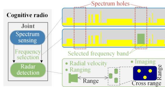
Fig. 12. Schematic diagram of the prototype's application in cognitive radio scenarios.
