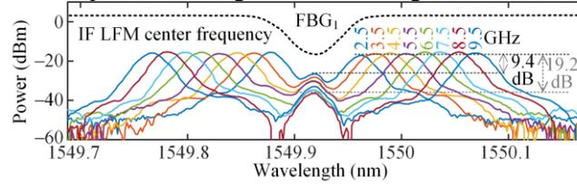
Fig. 2. Optical spectra of the optical LFM signal under different center frequencies of the IF LFM signal. The black dotted line shows the transmission spectrum of  $FBG_1$ .
