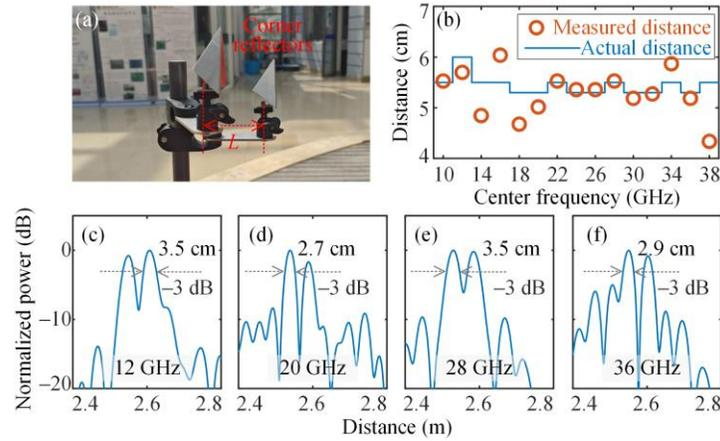
Fig. 5. (a) Photograph of the two smaller corner reflectors placed close to each other. (b) Measured distance between two smaller corner reflectors at different center frequencies. (c)-(f) Zoomed-in view of the de-chirped signal spectra at center frequencies of 12, 20, 28, and 36 GHz.
