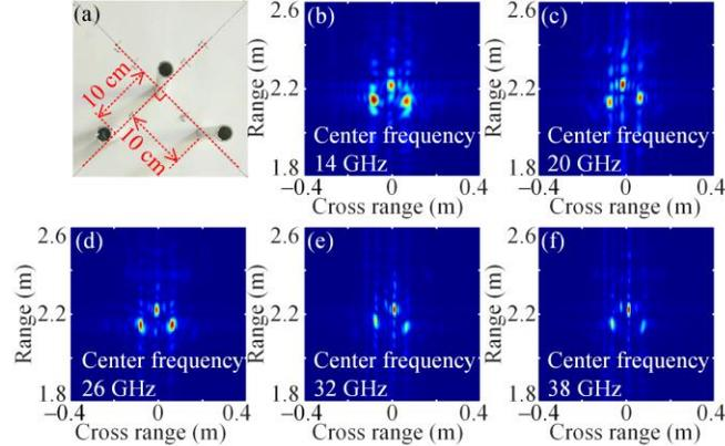
Fig. 8. (a) Photograph of three cylinders with an outer diameter of 2.5 cm for ISAR imaging. (b)-(f) ISAR imaging results obtained using the prototype operating at different center frequencies.
