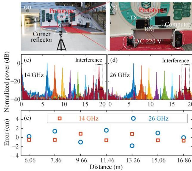
Fig. 4. (a) Photograph of the ranging experimental setup. (b) A zoomed-in view of the red-dotted rectangular area in (a). Ranging results of the corner reflector at different distances when the center frequencies of the LFM radar signal are (c) 14 GHz and (d) 26 GHz, respectively. (e) Ranging errors at different distances and center frequencies of the LFM radar signal.
