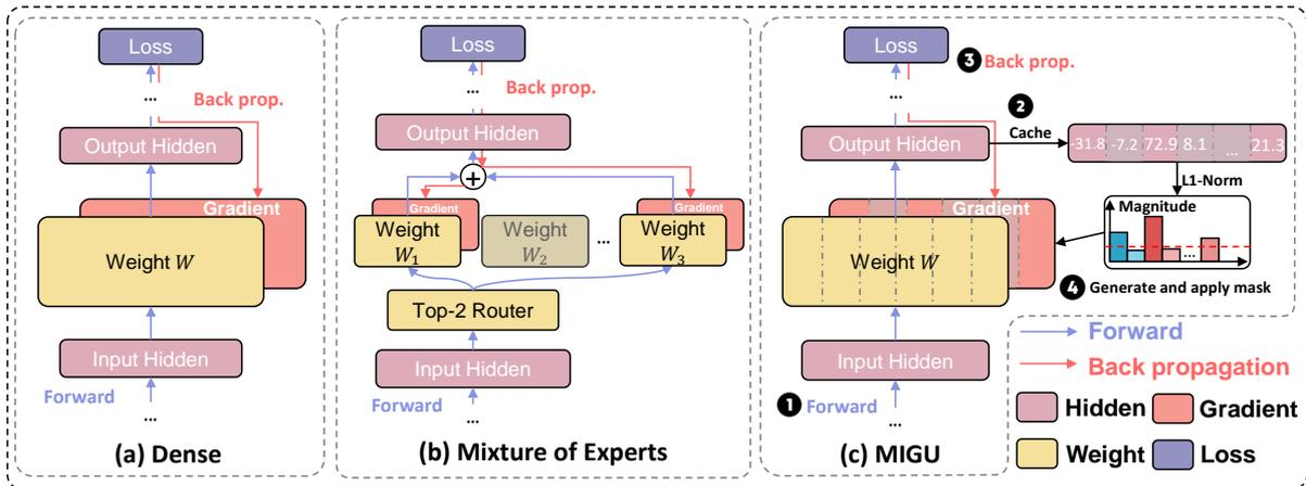
Figure 13: Differences between (a)Dense, (b)MoE and (c)MIGU
