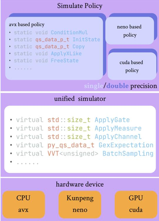
Figure III.1: The layer structure of the simulator. The *simulate policy* layer applies quantum gates to quantum states based on the current simulation hardware. The *unified simulator* layer uses different policies to complete the circuit simulation and expectation and gradient calculation. The *hardware device* layer shows that we support CPU, GPU and Kunpeng platform.
