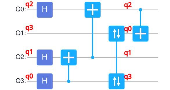
(c) A possible physical circuit. The initial mapping is `[3, 2, 0, 1]` and final mapping is `[1, 2, 0, 3]`.
