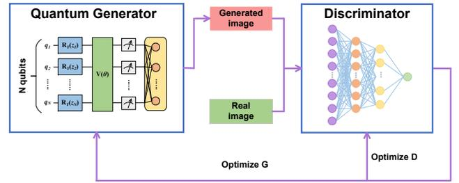
Figure V.13: The overall architecture and training process of QC-GAN.
