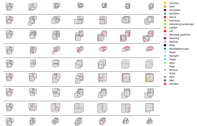
Fig. 27. Linear interpolation samples starting from the same latent code z of the learned latent space of a trained framework with edge-augmented encoder, vanilla VAE disentanglement module, MLP-based decoder, SVD embeddings, 25 categories of architectural elements, extra features of polygon vertices' coordinates, and boosted dimensions of the latent space
