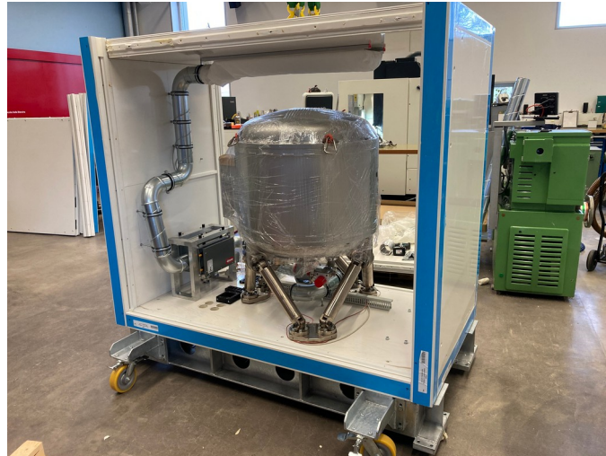
Figure 5: Photo of the thermal enclosure before closing. One also can see the vacuum tank.
