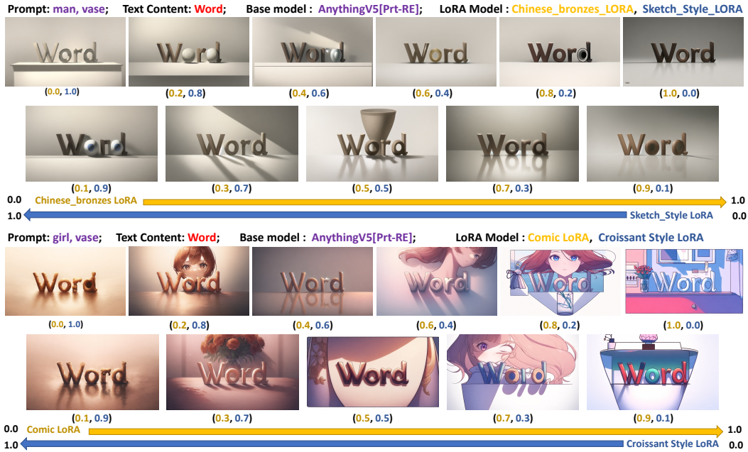
Figure 11: Impact of LoRA fusion with varying weights. Top: Merging Chinese Bronzes and Sketch Style LoRAs. Bottom: Combining Comic and Croissant Style LoRAs.
