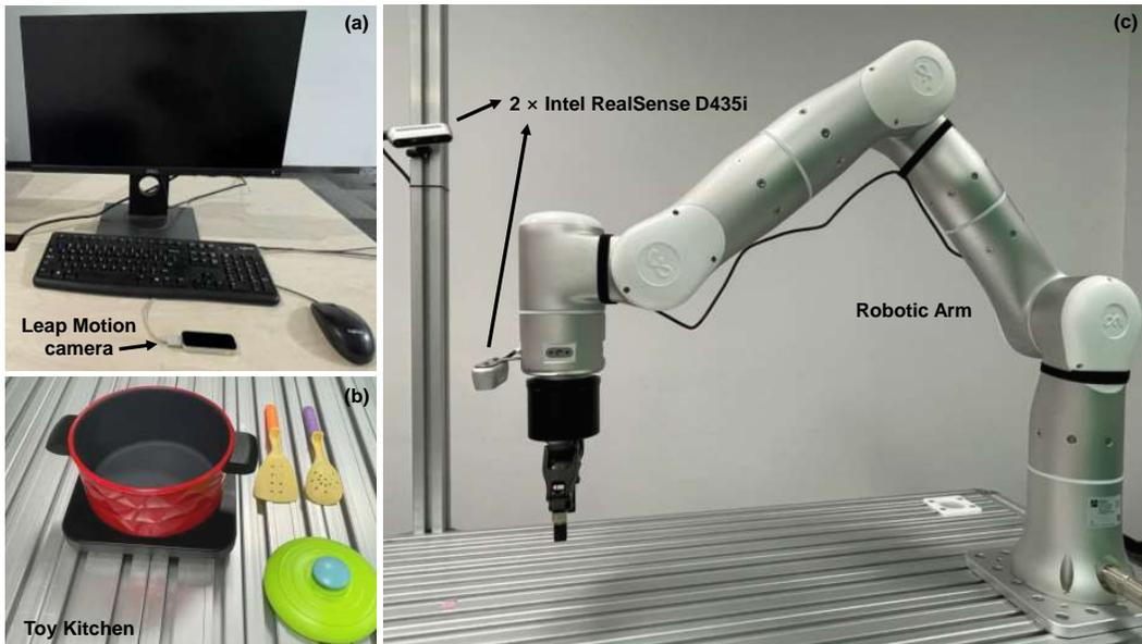
Figure 8: Realworld Pick-and-Place Experiment. The hardware setup comprises (a) a Leap Motion camera utilized for teleoperation data collection, (b) a toy kitchen environment set up for the pick-and-place task, and (c) a Flexiv Rizon4 robotic arm equipped with a gripper and two cameras. One camera is mounted on the wrist of the robotic arm, while the second one is positioned on the side.
