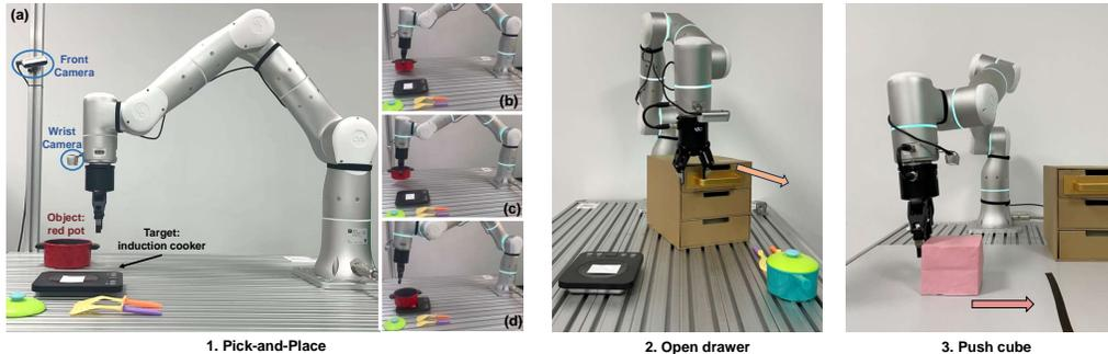
Figure 6: Real world setting. 1. *Pick-and-Place*: (a) Hardware setup. The robot gripper should pick the red pot up (b-c) and place it onto the black induction cooker (d). 2. *Articulated-Manipulation*: use a gripper to open the drawer. 3. *Push-cube*: use a gripper to push the cube across the line.
