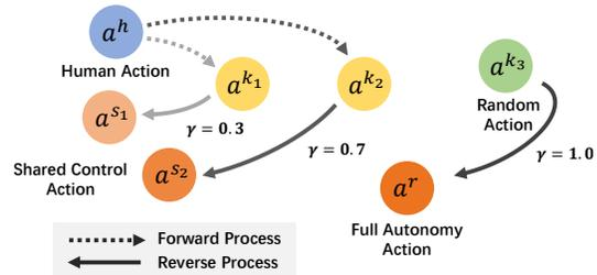
Figure 2: To achieve shared control between the human and agent, we blend the action from the human operator  $a^h$  using the forward and reverse processes. The parameter  $\gamma$  governs the control ratio, where a lower  $\gamma$  results in the action better aligning with the human operator’s intention. In contrast, a higher  $\gamma$  allows the learned agent to exert more influence over the blended action.
