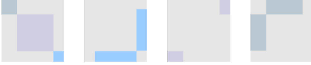
Figure 2: Schematic diagram of masks. The picture shows the masks of a trimer. The first mask on the left indicates whether the residues pairs are in the same chain. The colored part are intra-chain and the gray part are inter-chain. The three masks on the right indicate which two chains the residue pairs are located in when they are in different chains. For example, the dark blue part of the first mask on the right represents that the residue pairs come from the first and second chains respectively. For all masks, assign 1 to the colored parts and 0 to the gray parts.
