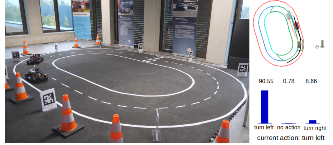
Fig. 1. Clockwise from the left: two ADAS model cars driving cooperatively, with the high-level decision being made by RL; real-time trajectory planning in the visualization; and the action distribution of the RL Agent after training.
