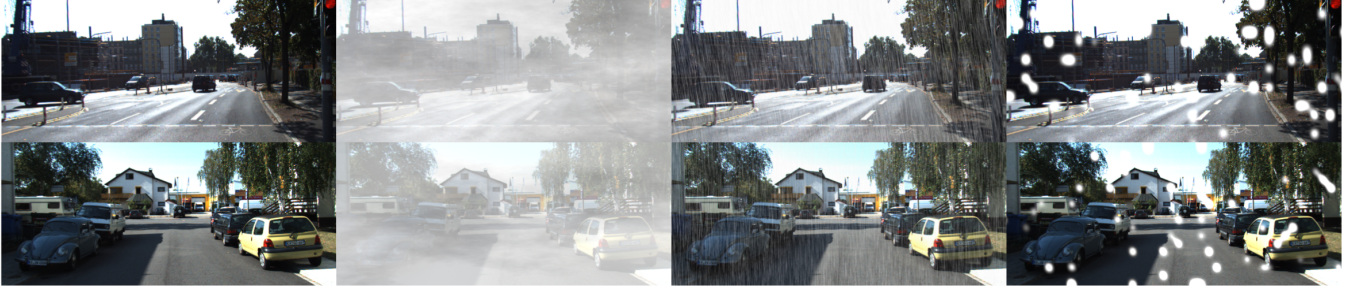
Fig. 5. Images from the KITTI dataset extended with image augmentations for adverse weather conditions. These images correspond to the high adversity validation sets. From left to right, in each column we show the base KITTI image, and the extreme fog, extreme rain, and extreme snow synthetic images respectively.
