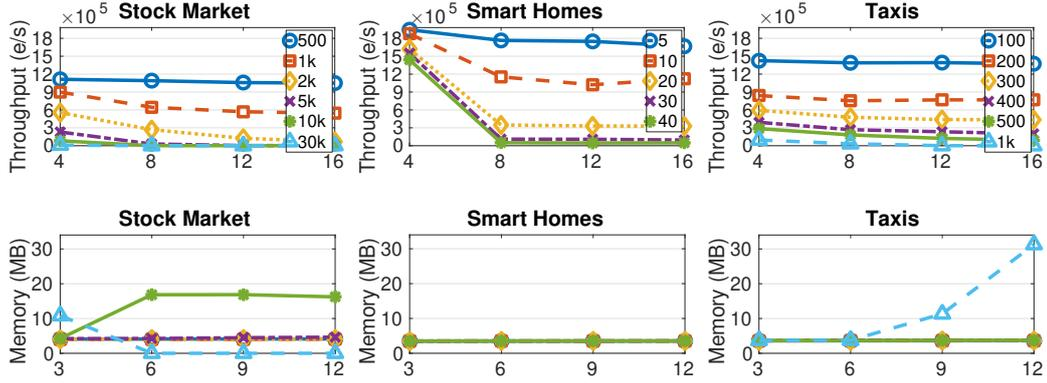
■ **Figure 9** Throughput and memory consumption for patterns with  $n$ -ary predicates and nested Kleene operators as a function of pattern length for various windows. SASE, FlinkCEP and Esper are excluded because they do not support patterns with nested Kleene operators.
