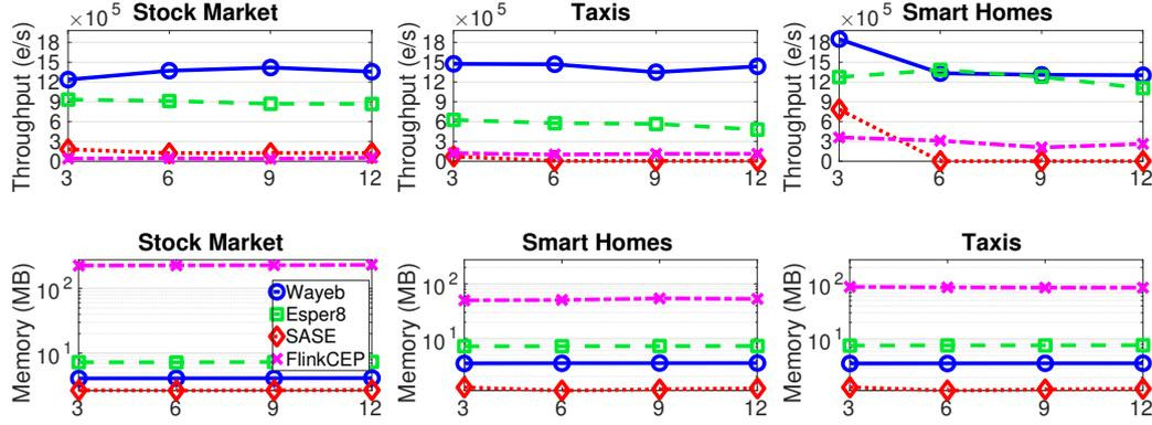
■ **Figure 6** Throughput and memory consumption for sequential patterns with  $n$ -ary predicates as a function of pattern length. Window sizes are  $w_{stock} = 500$ ,  $w_{smart} = 5$ ,  $w_{taxi} = 100$ .
