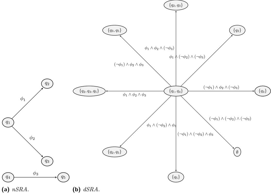
■ **Figure 14** Example of converting a *nSRA* to a *dSRA*.
