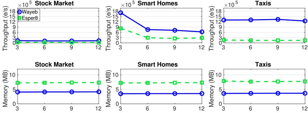
■ **Figure 8** Throughput and memory consumption for patterns with  $n$ -ary predicates and Kleene operators as a function of pattern length. SASE and FlinkCEP are excluded because they do not support patterns with Kleene operators with the expected semantics.
