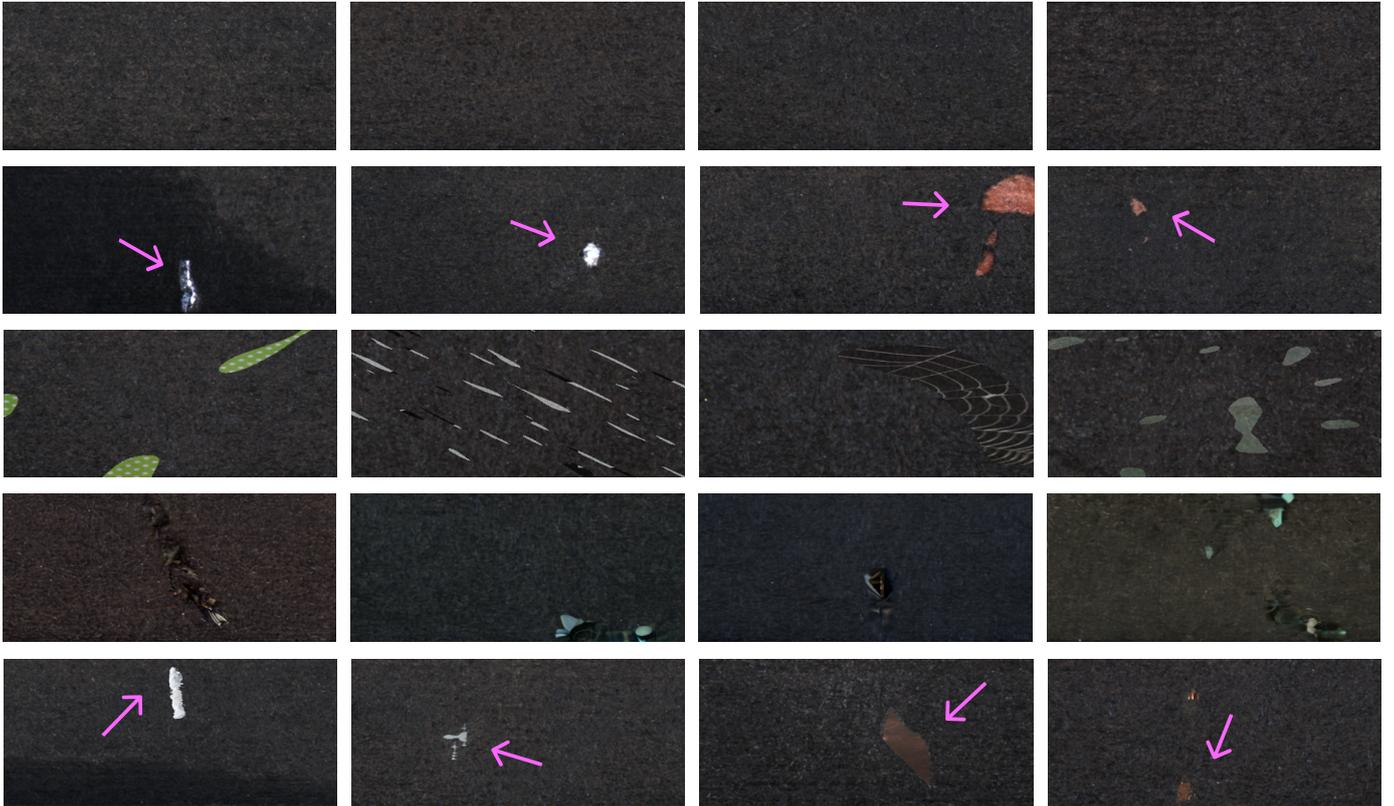
Fig. 2. First row displays some negative samples from the KSDD2 dataset. Instead, the second row shows some images of positive samples from the same dataset. In the third row, we show the MemSeg-generated defect samples. The fourth row shows In&Out generated defect samples. Lastly, the final row showcases images generated with DIAG. Notably, the defect images that DIAG generated are more realistic and in-distribution.
