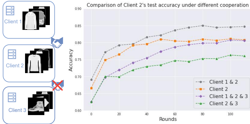
Figure 2: Toy examples show the importance of appropriate cooperation. Clients 1 and 2 have FashionMNIST datasets with labels \{4, 5, 6, 7\} , while Client 3’s dataset has labels \{0, 1, 2, 3\} . Using Client 2 as a baseline, accuracy comparisons indicate that collaboration between clients with similar data (Clients 1 and 2) is beneficial, whereas cooperation between clients with diverse data (Clients 2 and 3) is detrimental.
