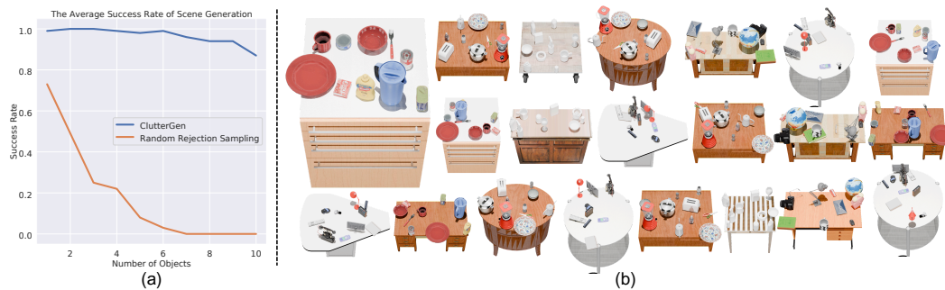
Fig. 1: (a) The success rate of generating a stable simulation setup. When the number of objects in the environment increases, the difficulty of creating such a stable setup also increases. The traditional heuristic method cannot create a simulation scene above 7 objects, while ClutterGen consistently achieves high success rates. (b) Diverse, cluttered, and stable simulation setups created by ClutterGen.
