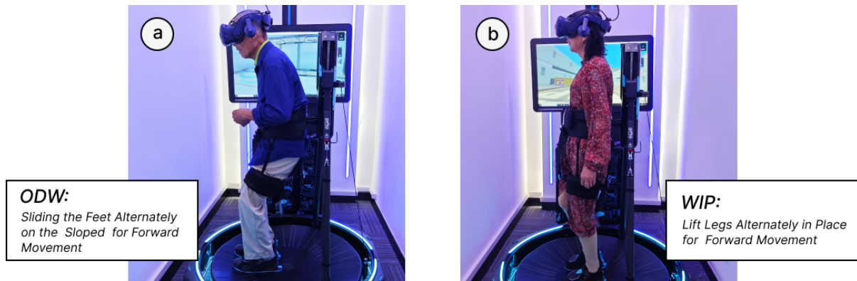
Fig. 2. Illustration of two walking locomotion modes: (a) omnidirectional walking (ODW) setup and (b) walking-in-place (WIP) setup.
