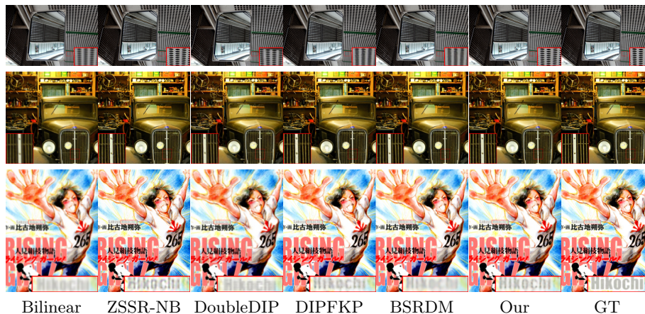
Fig. 2: Visualization of the synthetic images. Each row, from top to bottom, contains super resolved images from Urban100, DIV2K100 and Manga109, under the scale factor of 2, 3 and 4, respectively.
