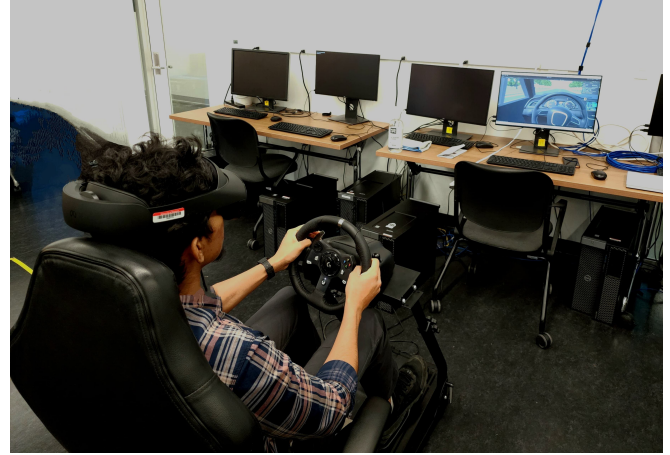
Fig. 1. Users engage in VR driving simulation using Meta Quest Pro VR and Logitech steering wheel, with the user's view displayed on the monitor and the HMD.
