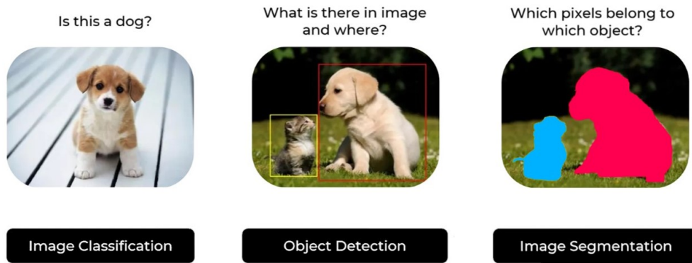
Fig. 21: Difference between image classification, detection and segmentation
