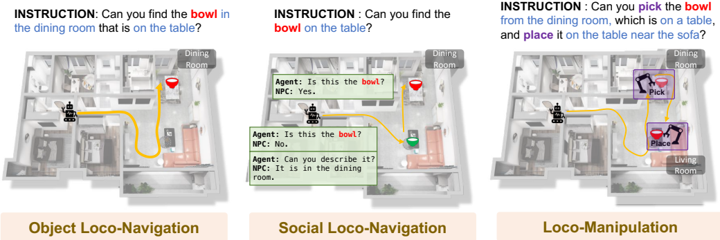
Figure 5: GRBench task examples. Three benchmarks are established for evaluating embodied agents: Object Loco-Navigation , Social Loco-Navigation , and Loco-Manipulation . The target object in the instruction are subject to some constraints generated by the world knowledge manager. Navigation paths , dialogues , and actions are depicted in the figure; please zoom in for better visualization.
