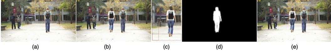
Figure 3: Post-processing to remove flickering square artifacts. a) Background image. b) Initial image generated from our pipeline. c) Zoomed-in view revealing artifacts around the inserted object. d) A trimap is generated to facilitate seamless blending of the object into the background. e) Post-processed frame showcasing the final result after blending the inserted object with the background.
