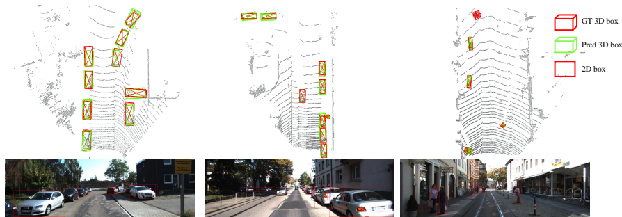
Fig. 5: Visualization of generated 3D boxes in bird’s eye view for outdoor scenarios.
