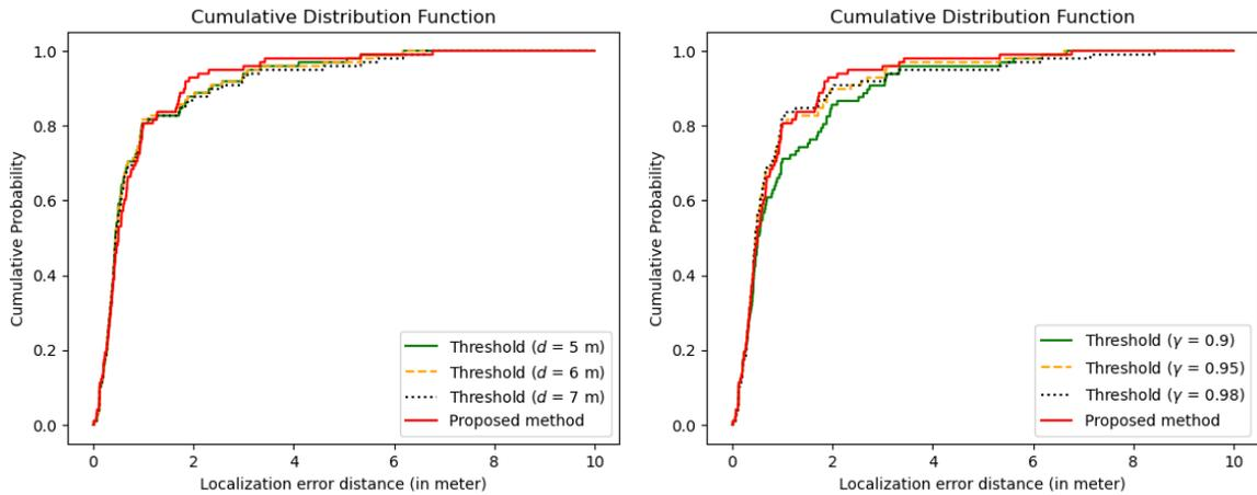
(a) CDF comparison with distance-threshold method (b) CDF comparison with probability-threshold method
