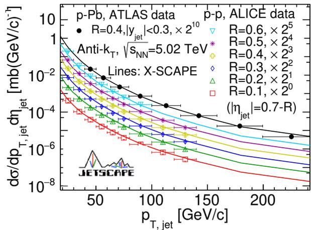
FIG. 5. The full jet  $p_T$ -differential cross sections at  $\sqrt{s_{NN}} = 5.02$  TeV for  $p$ - $p$  collisions with jet cone of radius  $R = 0.1$ – $0.6$  and 0–90%  $p$ - $Pb$  collisions with  $R = 0.4$ . The ALICE and ATLAS measurements are from [19, 75].
