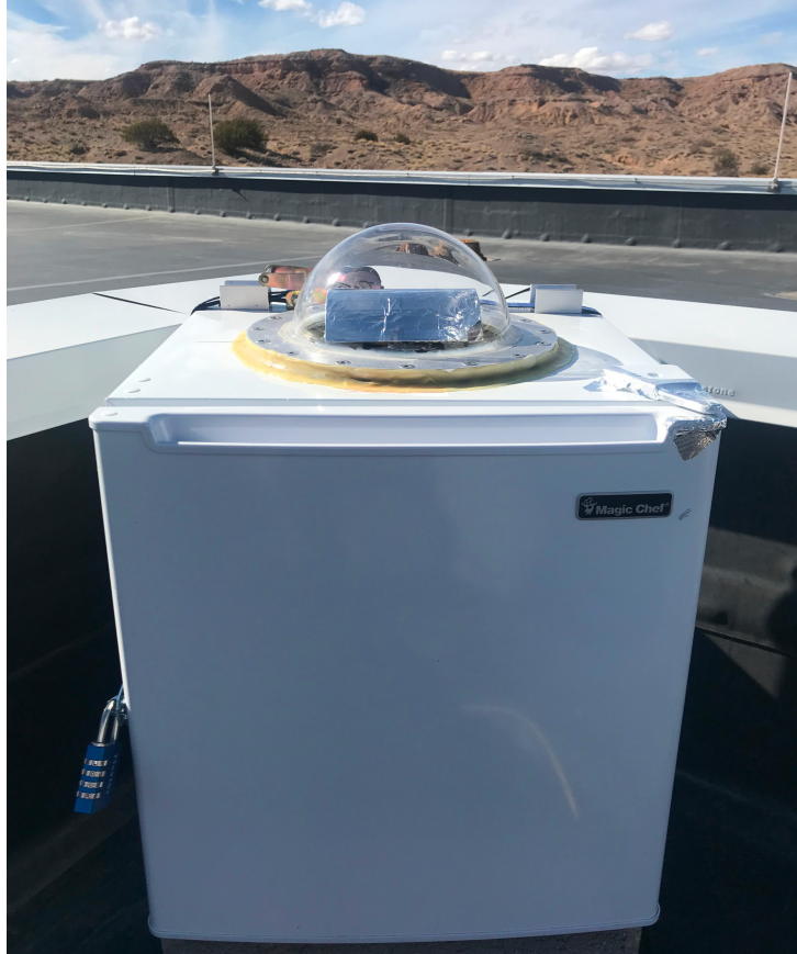
Figure 3. The deployed WiPT2 setup. All electronics are housed inside the minifridge; also seen are the clear plastic dome protecting the camera as well as the reflective clamshell sun shield within it.
