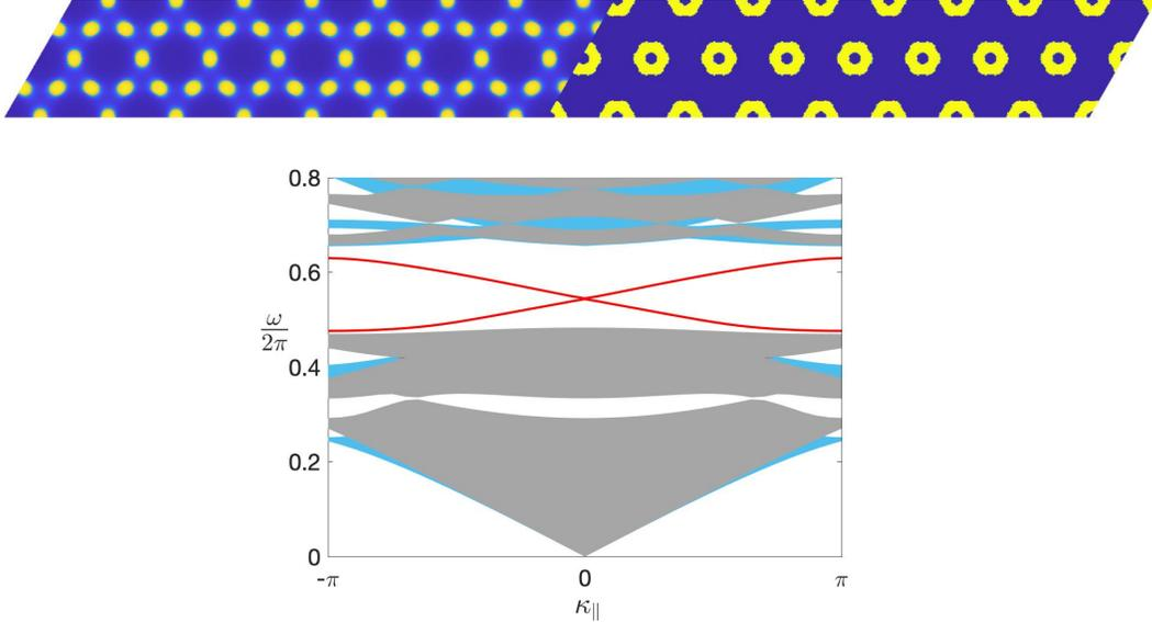
FIGURE 10. Top: The joint structure formed by two optimized periodic media that are shifted to the right with a distance of 0.025; Bottom: The dispersion relation of the edge modes along the interface for the wavenumber  $\kappa_{\parallel} \in [-\pi, \pi]$ . Two dispersion curves cross with each other when  $\kappa_{\parallel} = 0$ . See Section 4.3.
