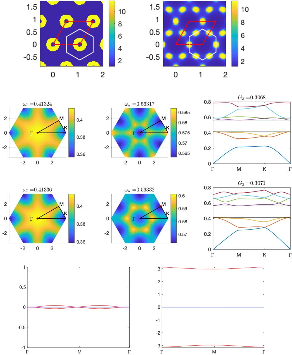
FIGURE 8. Row 1: Distribution of the electric permittivity for the optimized photonic crystals. Row 2-3: The third (left column) and fourth band (middle column) of two photonic crystals. The eigenvalues along the boundary of the reduced Brillouin zone  $\Gamma$ MK for two photonic crystals is plotted on the right column. Row 4: Wilson loops for the first three bands of the two optimized photonic crystals in Figure 8. The calculation for each band is the same as in Figure 7. See Section 4.3.
