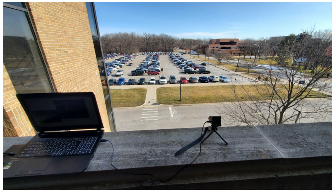
Figure 4: The data collection setup showing the hybrid event camera (DAVIS 240) mounted on a tripod at the edge of a building overlooking the street and part of the parking lot. A laptop adjacent to the camera setup is used for data recording and sensor control.
