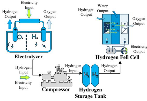
**Figure 1:** Schematic diagram of hydrogen storage system.
