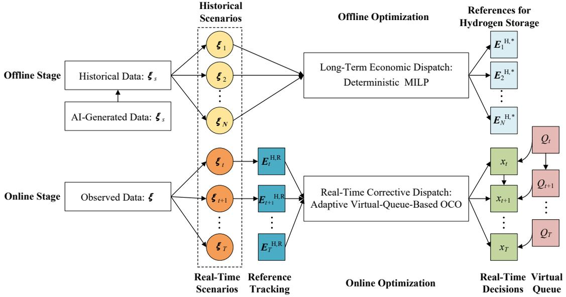
Figure 5: Diagram of prediction-free two-stage coordinated optimization framework.
