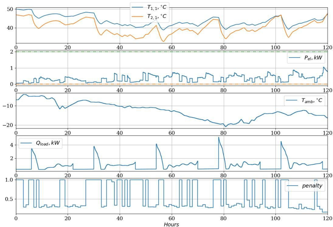
**Figure 14:** Simulation results of the MPC using optimal penalty signal. The top panel shows the water temperature of the top and bottom of the tank. The second panel demonstrates the electricity consumption. The ambient temperature is provided in the third panel. The requested load of the tank and the optimal penalty signal are shown in the fourth and fifth panels, respectively.
