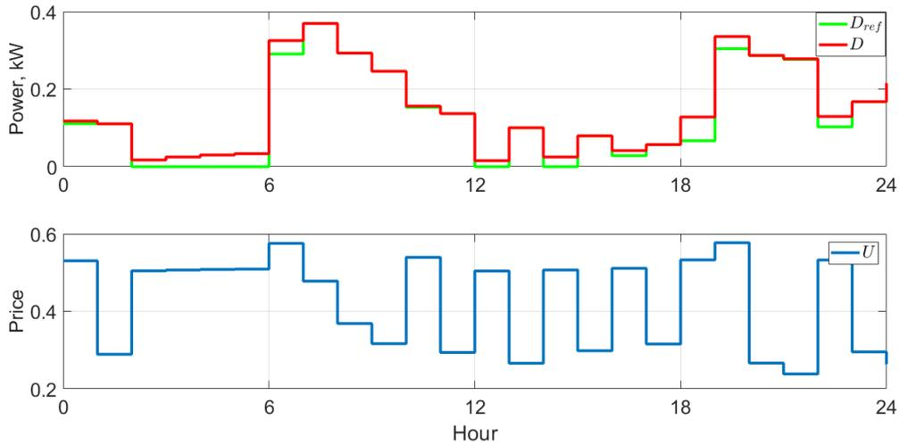
**Figure 8:** Simultaneous optimal price generation with absolute value objective function. The top panel shows the reference and the actual demand for 24 hours. The bottom panel shows the optimal price signal.
