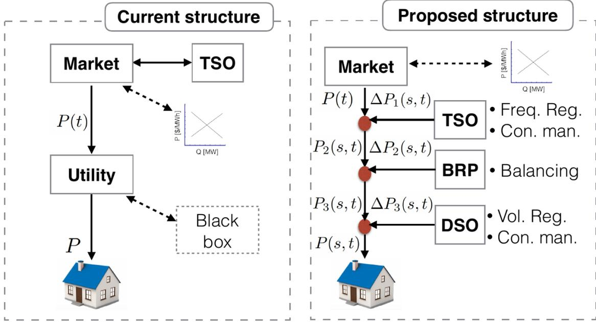
**Figure 5:** The existing vs. novel structures for the price generation considering ancillary services. The supply and demand curve is shown as a tool for electricity market price determination, where  $P$  is the price per MWh and  $Q$  is the supply power.
