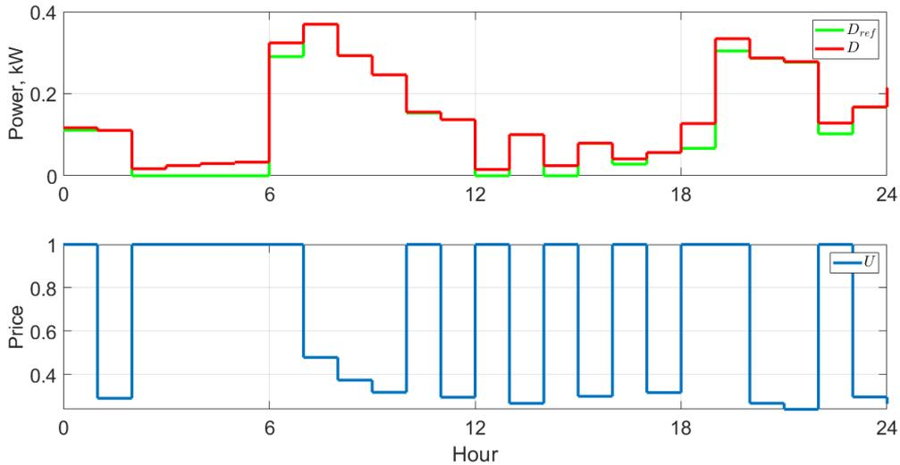
**Figure 6:** Sequential optimal price generation with absolute value objective function. The top panel shows the reference and the actual demand for 24 hours. The bottom panel shows the optimal price signal.
