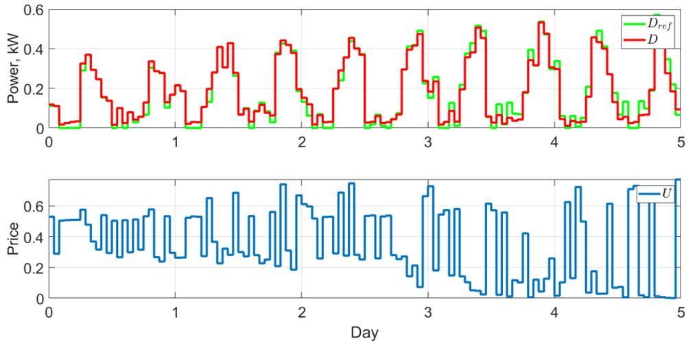
**Figure 9:** Simultaneous optimal price generation with absolute value objective function. The top panel shows the reference and the actual demand throughout five days. The bottom panel shows the optimal price signal.
