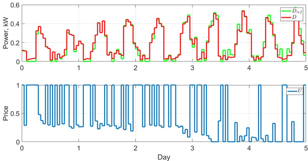
**Figure 7:** Sequential optimal price generation with absolute value objective function. The top panel shows the reference and the actual demand throughout five days. The bottom panel shows the optimal price signal.
