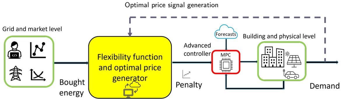
Figure 3: Block diagram of higher and lower levels of smart energy OS in the presence of FF.
