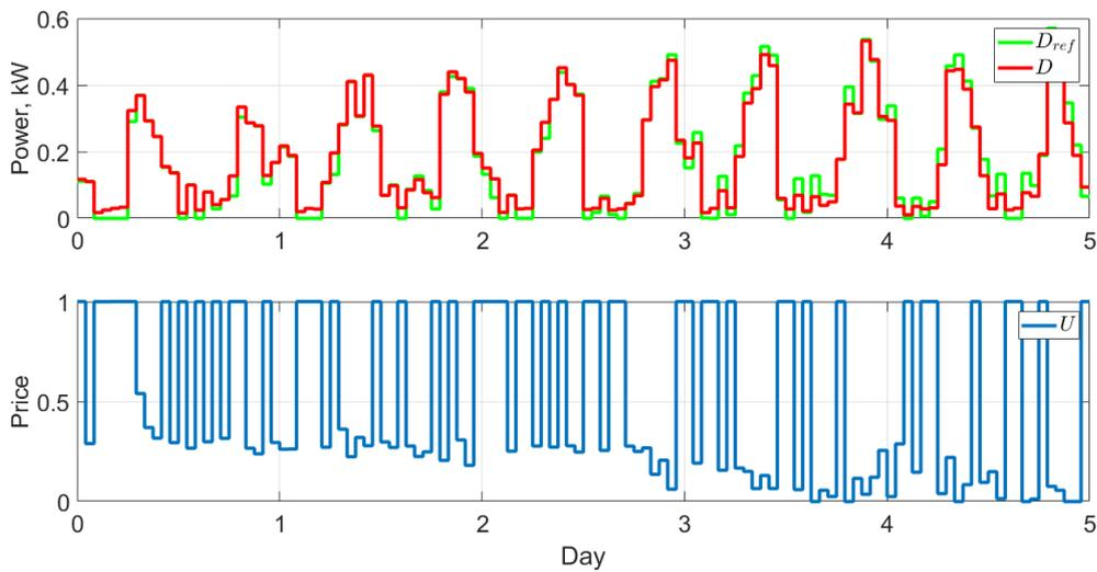
**Figure 13:** Simultaneous optimal price generation with quadratic objective function. The top panel shows the reference and the actual demand throughout five days. The bottom panel shows the optimal price signal.
