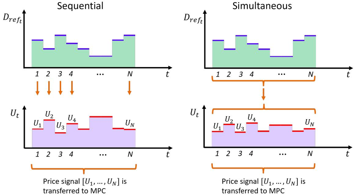
Figure 4: Sketch of sequential and simultaneous price signal generation in the Smart Energy OS based on FFs. For given price signals,  $U_t$  or  $[U_1, \dots, U_N]$ , the flexibility function is used to predict the demand,  $D_t$  or  $[D_1, \dots, D_N]$ , which should be as close as possible to the reference demand,  $D_{ref_t}$  or  $[D_{ref_1}, \dots, D_{ref_N}]$ .
