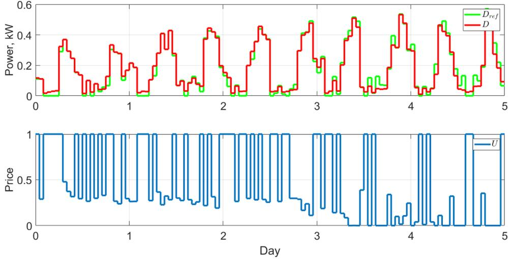
**Figure 11:** Sequential optimal price generation with quadratic objective function. The top panel shows the reference and the actual demand throughout five days. The bottom panel shows the optimal price signal.
