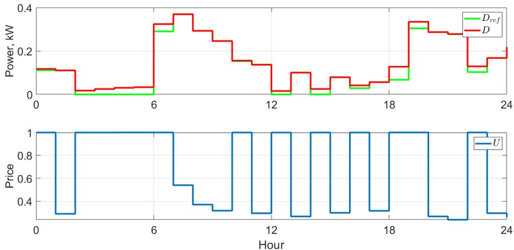
**Figure 12:** Simultaneous optimal price generation with quadratic objective function. The top panel shows the reference and the actual demand for 24 hours. The bottom panel shows the optimal price signal.
