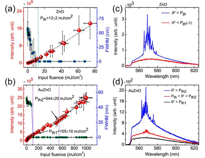
FIG. 3. Lasing threshold characteristics (a) and (b), and emission spectra at different input fluences (c) and (d) for ZnO and AuZnO, respectively.  $P_{th}$  refers to the lasing threshold of the systems and  $IF$  is the input pump fluence.
