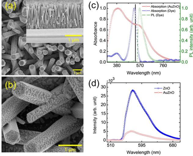
FIG. 2. (a) FESEM image of top-view of Au NI decorated ZnO NRs. The inset shows the cross sectional view of ZnO NRs. (b) A magnified view of Au NIs on ZnO NRs. (c) Extinction spectra of AuZnO, absorption and PL spectra of Pyrromethene-doped PMMA. The solid black line indicates the pump laser wavelength. (d) PL spectra of Pyrromethene-doped PMMA coated ZnO and AuZnO samples.
