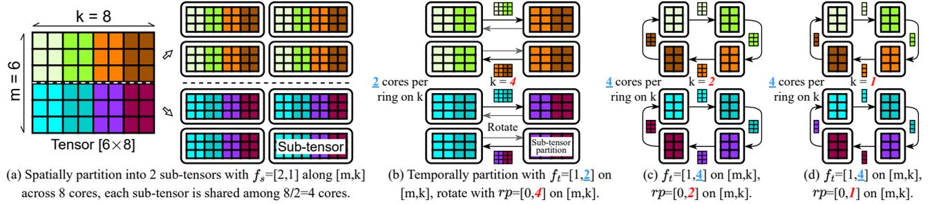
Figure 6. Illustration of  $r$ Tensor partitioning and rotating.
