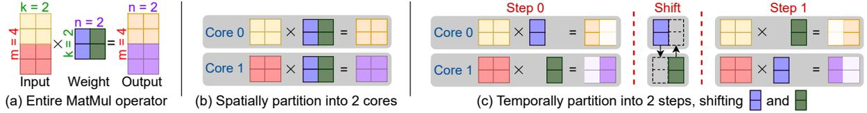
**Figure 3.** An example that maps a MatMul operator to two cores with the compute-shift style execution. Both (b) and (c) are valid compute-shift execution plans, but with different tradeoffs between memory footprint and communication overhead.
