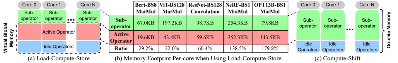
**Figure 2.** A comparison of the conventional load-compute-store (a) vs. our compute-shift (c) style execution. (b) shows the per-core memory footprint of representative operators when running DNN models on IPU using VGM. **Ratio** is the potential increase in sub-operator size by removing VGM. The result of OPT13B [57] comes from profiling one of its layers on IPU.
