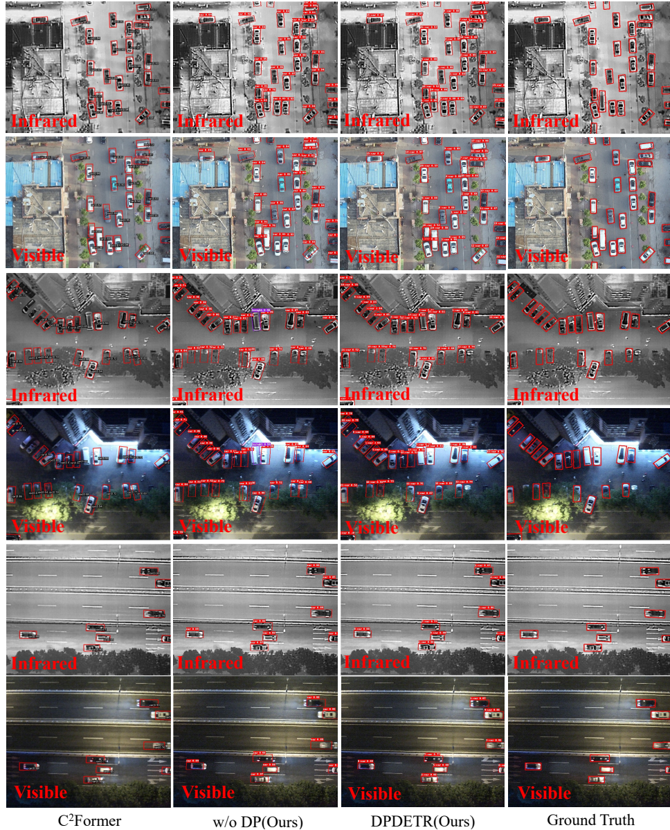
Fig. 8. Detection Results on the DroneVehicle Dataset. The w/o DP method represents without decoupled position and only uses infrared modality annotations to constrain. The confidence threshold is set to 0.5 when visualizing these results.
