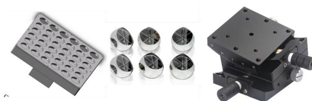
Figure 11 The experimental CCR array (the left image shows the 6 \times 6 array of CCRs used in the experiments, the middle image depicts a single CCR, and the right image displays the manually adjustable tilt table that is capable of adjusting angles in two directions).
