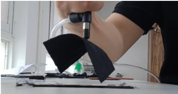
Dia. 5. Photo of single grabbing test to determine the grabbing pressure and radius of vacuum grabbing pressure theoretical circle.
