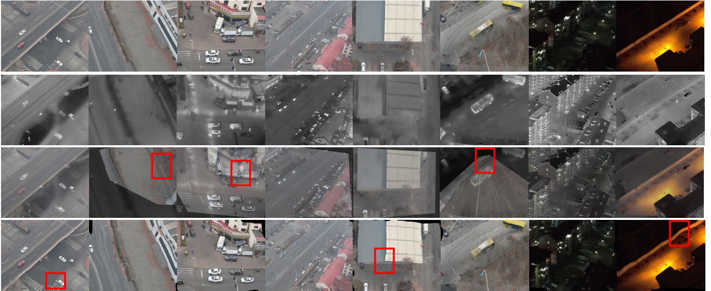
Fig. 5: Comparison of registration results using LoFTR and SuperFusion under different viewpoints and lighting conditions. The first and second rows present the RGB and TIR channel images, respectively. The third and fourth rows showcase the registration outcomes of the LoFTR and SuperFusion methods. Regions with significant registration discrepancies are highlighted.
