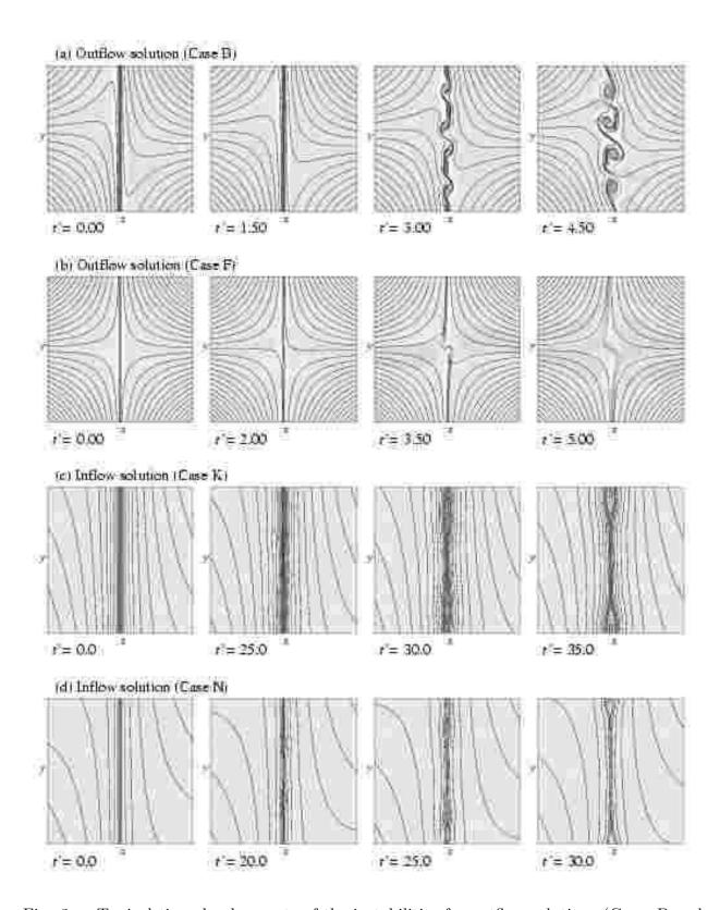
Fig. 3.— Typical time developments of the instabilities for outflow solutions (Cases B and F) and inflow solutions (Cases K and N). Solid lines represent the magnetic field lines. Gray scale represents the z-component of the current density; darker gray corresponds to a larger current density. The displayed area is |x| < 2, |y| < 2 (the origin is at the center).
