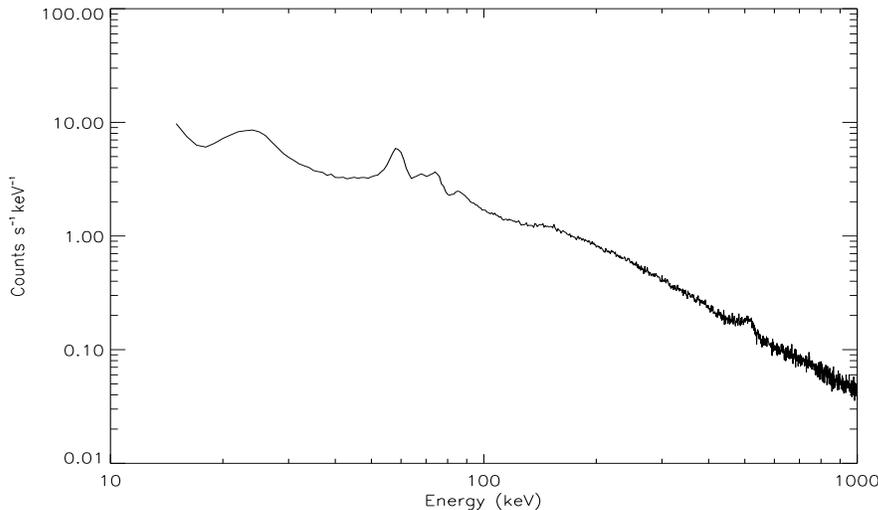
Fig. 1. ISGRI Background Spectrum obtained from a science window sample (acquired during the revolution 53); the exposure time is 1800 seconds. The 511 keV line component is clearly visible. The lines below 100 keV are due to lead and tungsten fluorescence in the telescope.
