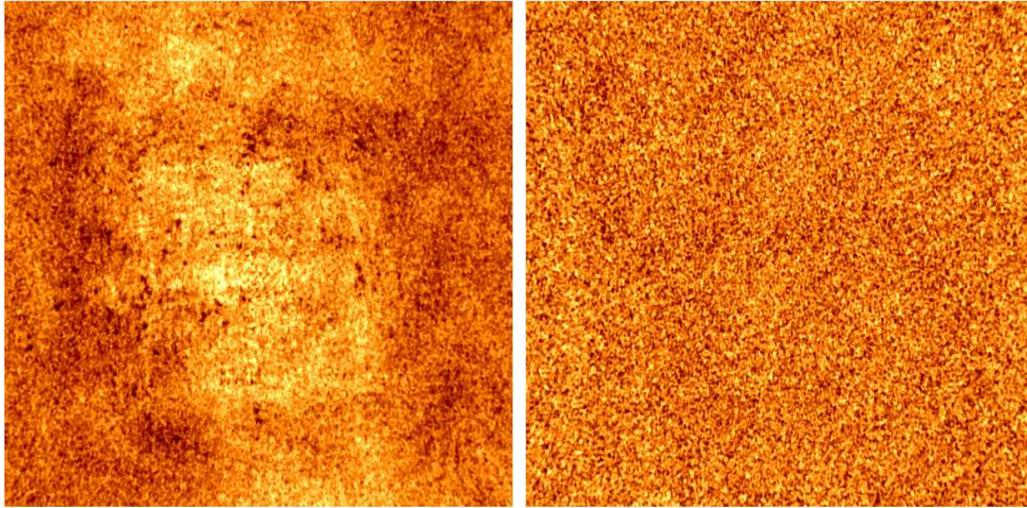
Fig. 3. The standard processing of the GCDE ISGRI data has not shown any evidence for 511 keV point sources. The image on the left shows the mosaic in the energy band 485 keV - 535 keV. The large structure that appears is due to the overlap of the dithering points. After the correction for these effects (image on the right panel), the systematic structures in the image are strongly reduced
