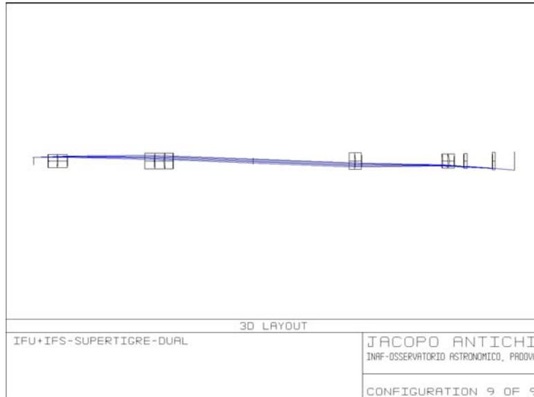
**Figure 5: Sketch of the IFS system: the adopted glasses are S-FTM16 and CAF2, the total length < 1.5 m.**
