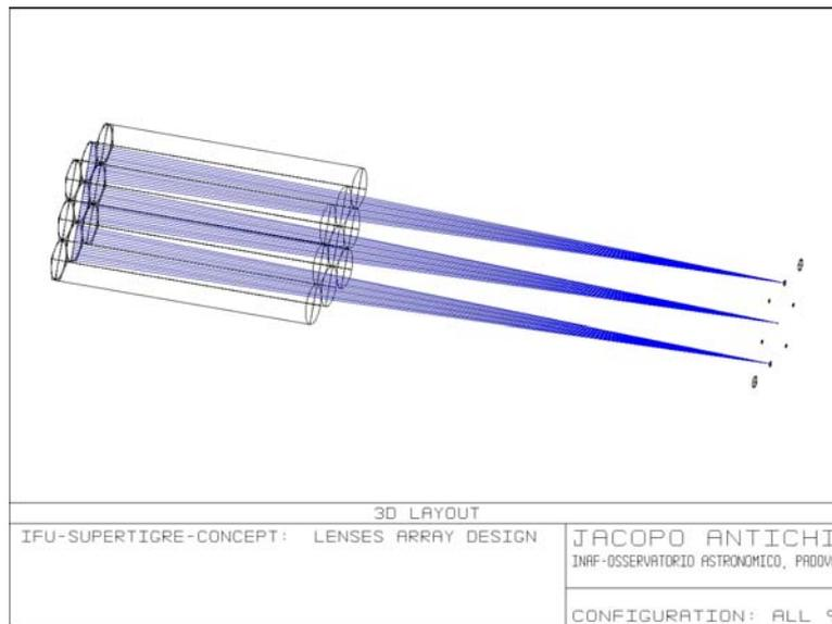
Figure 4: Sketch of the IFU-system: the adopted glass is BK7; the pitch is  $150 \mu\text{m}$  and the shape hexagonal.
