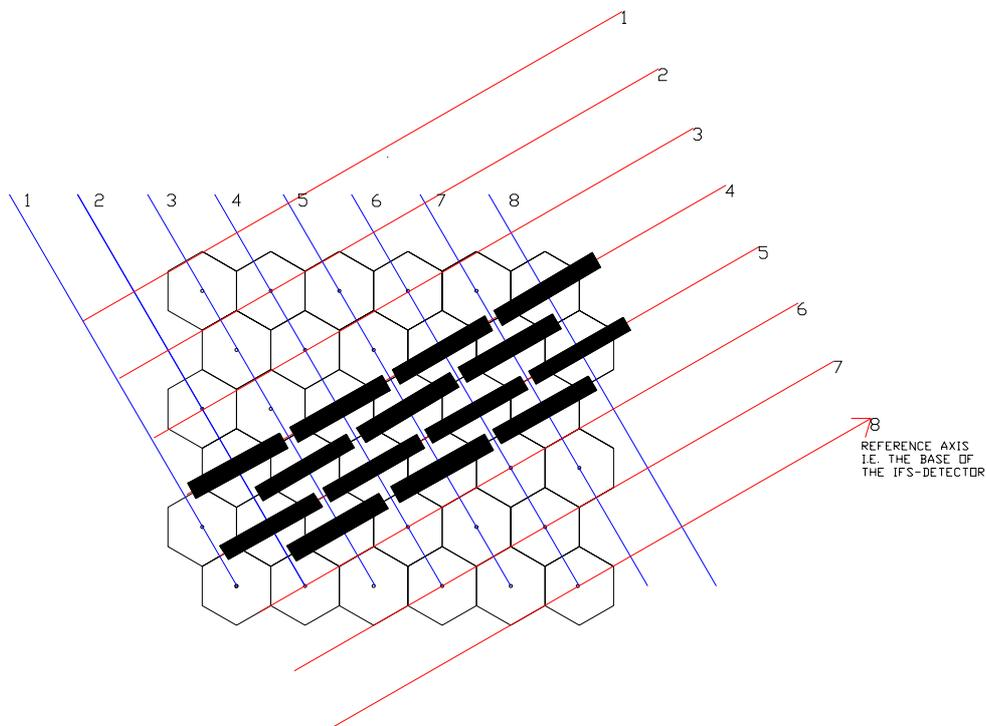
**Figure 1: Thin hexagons represent the microlens array (IFU). Solid rectangles represent the arrangement of the spectra on the IFS focal plane. Oblique rows and columns represent the orientation of the IFS Detector**
