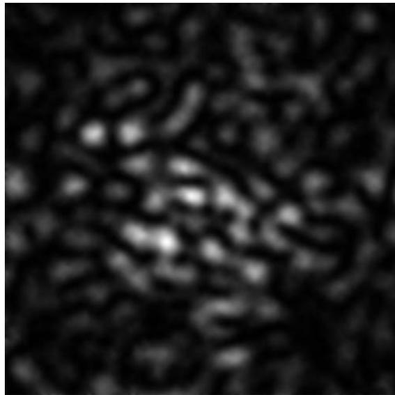
**Figure 2: Example of simulated speckle pattern residual (0.5 msec integration time) after Adaptive Optics correction on a lenses-array with specifications matching the ones described in the text.**
