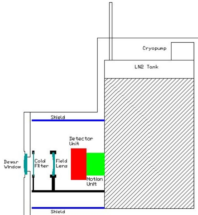
**Figure 6: A sketch of the IFS cryostat in which the LN2 tank is perpendicular to the direction of the optical path**
