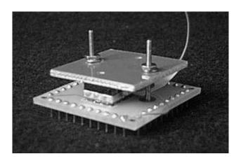
**Figure 3.** The assembled flip-chip CZT detector. The top cover (G10 material) holds the CZT between conductive rubber pads for readout and application of bias voltage.
