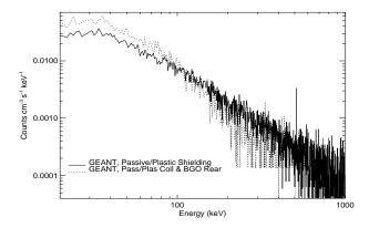
Figure 9. Expected gamma-ray backgrounds per area expected for the CZT/BGO detector with passive/plastic collimator and pixellated flip-chip detectors with passive/plastic shielding, as computed by GEANT. The PoRTIA and WUSTL/UCSD results are reproduced as in Figure 1. The thicker pixellated detectors record a higher background per area.
