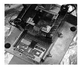
Figure 7. The passive/plastic collimator shown in the flight configuration with the tiled flip-chip detector assembly. The collimator surrounds the detector carrier board, which is plugged into the VA-TA board. The ASICs are mounted under the black rectangular cover to the lower left. The rear passive/plastic shield (not shown) will lie directly beneath the VA-TA board.
