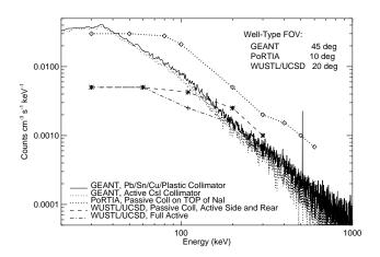
**Figure 1.** GEANT simulations of CZT detectors with active and passive/plastic collimators and an active rear shield, compared with previous measurements made using active rear shields and active or passive collimators. Spectra are plotted per volume to account for differing detector thicknesses. The fields of view are 45° for the GEANT simulations, 10° for PoRTIA, and 20° for the WUSTL/UCSD experiment.
