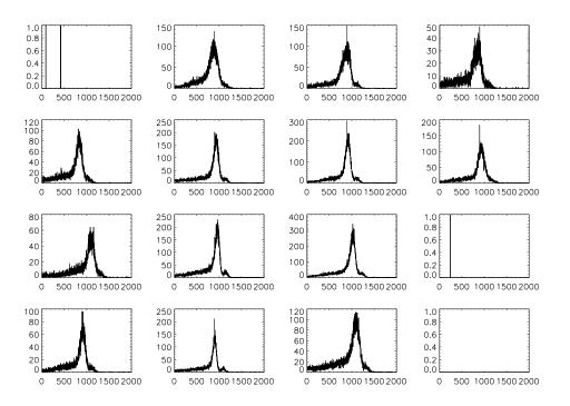
**Figure 8.** "First light"  $4 \times 4$  array of  ${}^{57}$ Co spectra taken with the IMARAD Au/In detector mounted on the flip-chip carrier card read out by the VA-TA ASIC. Three pixels were found to be disconnected because the conductive rubber pads had become detached. The pixels in the top row are unusually noisy, either due to bad contact with the pixels or noise in certain ASIC channels.
