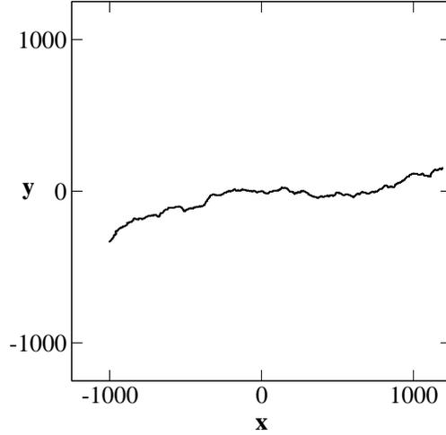
FIG. 2: A typical backbone of the fracture pattern. This is the projection onto the x-y plane of the experimentally observed boundary between the two parts of the material that separate when the fracture pattern hits t
