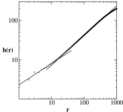
FIG. 3:  $h(r)$  averaged over all the backbone and over 70 fracture patterns each of which of 10 000 fracture events. There is a cross-over between a scaling law with roughness exponent  $0.54 \pm 0.05$  to and exponent of  $0.75 \pm 0.02$
