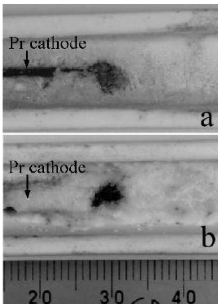
FIG.1. Photograph of deposits (dark areas around the centers) prepared from (a) KCl-bath and (b) NaCl-bath. The scale in unit of mm is shown at the bottom.
