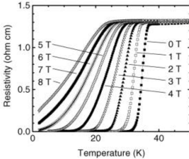
FIG.2. Electrical resistivity plotted against temperature for the sample prepared from the NaCl-bath. Applied magnetic fields were changed between 0 and 8 T with the increment of 1 T, each of which is shown in the figure.
