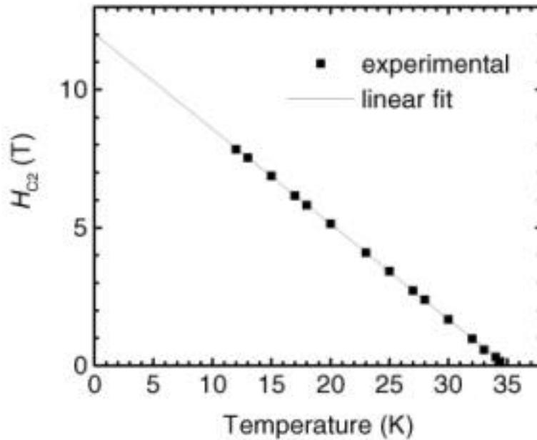
FIG.3. Upper critical field ( $H_{C2}$ ) plotted against temperature ( $T$ ), which was determined from the resistivity data (FIG. 2). Linear extrapolation of the experimental data is shown as linear fit.
