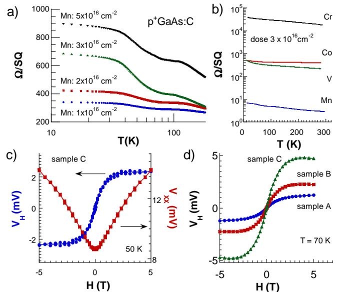
FIG. 1: a) Sheet resistance( $\Omega$ /SQ) as function of temperature (T) for samples A - D. b)  $\Omega$ /SQ as function of T for Co, Cr, Mn, V implanted p $^{+}$ GaAs:C with 3  $\times 10^{16}$  cm $^{-2}$  dose. c) AC magneto-transport measurement of sample C at 50 K with excitation current of 100  $\mu$ A. d) AC Hall Effect measurement of samples A - C at 70 K.
