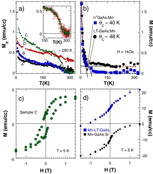
FIG. 2: a)  $M_R$  as a function of temperature ( $T$ ) for Mn implanted  $p^+$ GaAs:C (near  $T_C$  for Sample C, inset). b) Magnetization ( $M$ ) as a function of  $T$  for sample X and Y with Curie-Weiss Law fit.  $M$  as a function of applied field at 5 K for sample C (c) and sample X and Y, offset for clarity (d).
