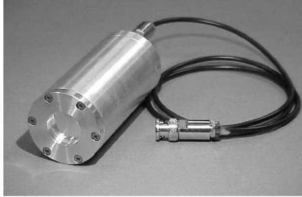
Figure 5: A photodiode-based detector used for measuring DAFS spectra. The dimensions are the same as for common scintillator-based detectors, allowing the use of off-the-shelf detector mounts.
