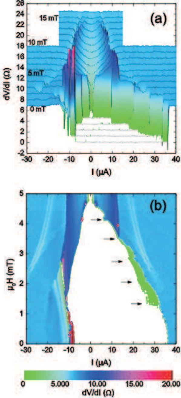
FIG. 3: (Color online) (a) measured differential resistance  $dV/dI$  as a function of the dc current for different magnetic fields measured at  $T = 1.100$  K. The curves for non-zero field are shifted for clarity. A color map surface is given for comparison with (b). (b) contour plot of the differential resistance  $dV/dI$  as a function of dc current and magnetic field measured at  $T = 1.100$  K for low magnetic fields. The arrows indicate the points where the vorticity changes.
