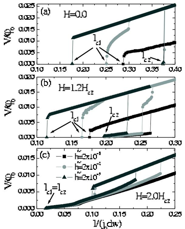
FIG. 7: Current-voltage characteristics of the superconducting square with contacts calculated for different heat removal coefficients  $\tilde{h}$  and magnetic fields. Current is normalized by the value  $j_0dw$ , where  $d$  and  $w$  are the lead thickness and width, respectively.
