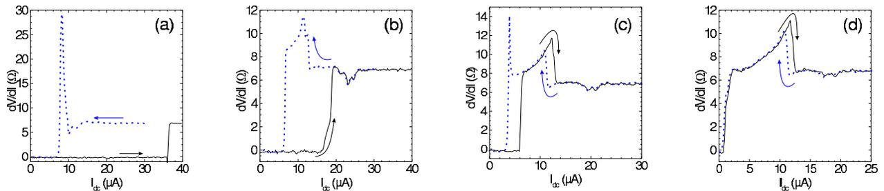
FIG. 2: Measured  $dV/dI$  as a function of the dc current at (a)  $\mu_0 H=0$  mT, (b)  $\mu_0 H=3.2$  mT, (c)  $\mu_0 H=4.2$  mT and (d)  $\mu_0 H=5$  mT measured at  $T = 1.100$  K. The full black and dashed blue lines are for increasing and decreasing current, respectively.
