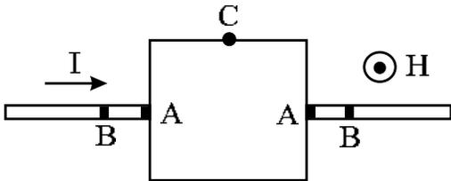
FIG. 4: Model geometry. Between points A and B phase slip centers appear at  $H \lesssim H_{c2}$ . In point C we trace out the dependence of  $|\psi|$  on the magnetic field (see text below and Fig. 5).
